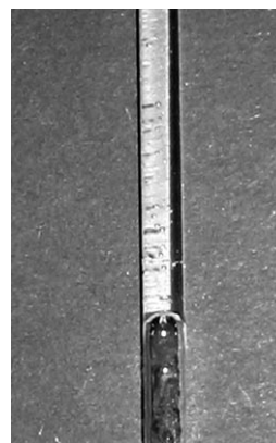
Figure 5. At mM concentrations receptor 2 caused gelation of an aqueous solution during attempts to perform NMR titrations in \text{D}_2\text{O} .
